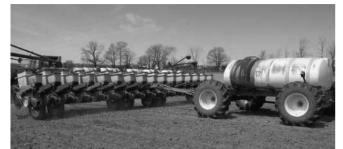
Figure 1. Dunlogon Farms of Stayner Ontario can bring 1,600 gallons of UAN (32%) in a tow-behind cart in their attempts to keep application costs low and N losses minimized. N is banded 6 inches off the row on the corn planter.
